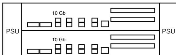
In a single-chassis HA pair, both controllers are in the same chassis. The HA interconnect is provided by the internal backplane. No external HA interconnect cabling is required.
