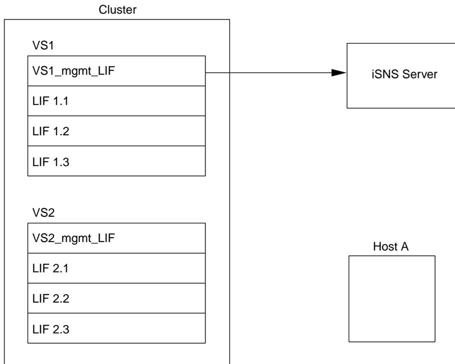
In the next example, after the iSNS server completes the registration with the target, Host A can discover all the LIFs for VS1 through the iSNS server as indicated in step 1. After Host A completes the discovery of the LIFs for VS1, Host A can establish a connection with any of the LIFs in VS1 as shown in step 2. Host A is not aware of any of the LIFs in VS2 until the management LIF VS2\_mgmt\_LIF for VS2 registers with the iSNS server.
