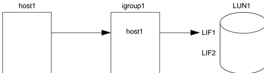
You can limit access to LUN1 by using a port set. In the following example, initiator1 can access LUN1 only through LIF1. However, initiator1 cannot access LUN1 through LIF2 because LIF2 is not in port set1.
