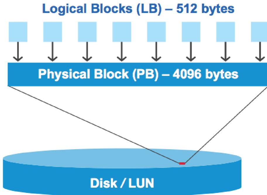
The host operating system can begin a read or write I/O operation at any logical block. I/O operations are only considered aligned when they begin at the first logical block in the physical block. If an I/O operation begins at a logical block that is not also the start of a physical block, the I/O is considered misaligned. ONTAP automatically detects the misalignment and reports it on the LUN. However, the
