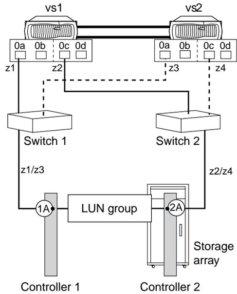
The initiator ports 0a of controllers vs1 and vs2 are connected to the storage array port 1A and ports 0c of the controllers are connected to the storage array port 2A.
