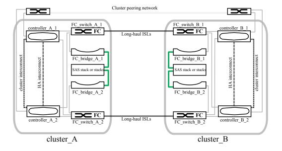
The following illustration shows a more detailed view of the connectivity in a single MetroCluster cluster (both clusters have the same configuration):
