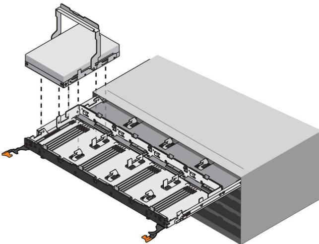
4. Lower the drive straight down, and then rotate the drive handle down until the drive snaps into place under the drive release lever.
