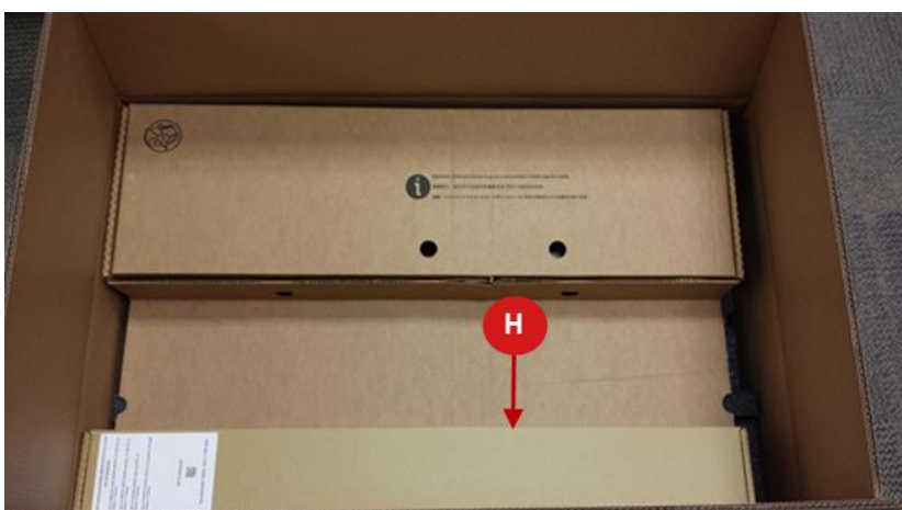
H. Add Rail Kit (if rail kit is being returned) or spacer box (provided)
