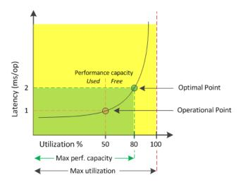
The *operational point* identifies that the aggregate is currently operating at 50% utilization with latency of 1.0 ms/op. Based on the statistics captured from the aggregate, Unified Manager determines that additional performance capacity is available for this aggregate. The *optimal point* is identified as the point when the aggregate is at 80% utilization with latency of 2.0 ms/op. Therefore, you can add more volumes and LUNs to this aggregate so that your systems are used more efficiently.
