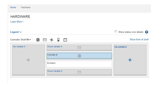
From the back of the shelf, you can view the E2800 controller, the power and fan canisters in the appliance, the battery in the E2800 controller, and component temperatures.
