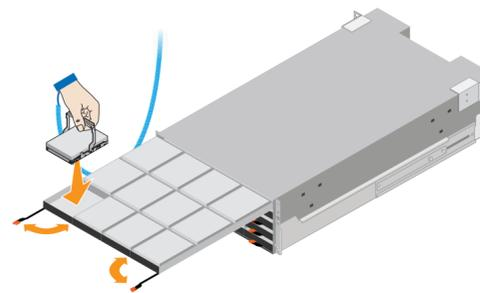
**ATTENTION: Risk of equipment damage** — Stop pushing the drawer if you feel binding. Use the release levers at the front of the drawer to slide the drawer back out. Then, carefully reinsert the drawer into the slot.
