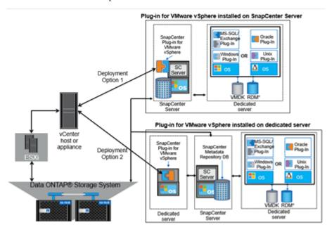
\*RDM is not supported for backups of VMs or datastores using the web client GUI in vCenter. However, RDM is supported for application-consistent backups using other SnapCenter plug-ins (for example, backups of Microsoft SQL Server or Oracle databases residing on RDMs).
