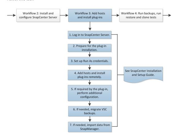
Use the SnapCenter Add Host wizard to add hosts and install the plug-ins packages. The plug-ins are automatically installed on the specified remote hosts.
