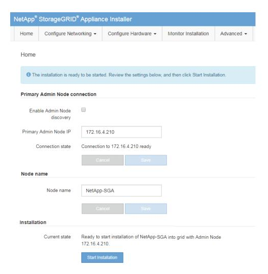
2. In the Primary Admin Node connection section, determine whether you need to specify the IP address for the primary Admin Node.
