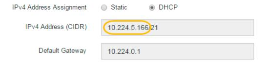
**5.** Optionally, set a static IP address for the E2700 controller management port.
