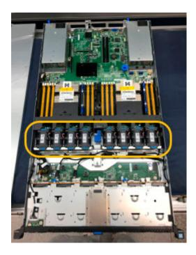
5. Lift the failed fan out of the chassis.
