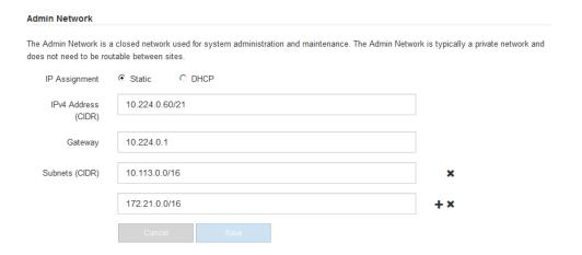
When you configure the Admin Network, you specify the IP address, gateway, and subnets used for Management Port 1 on the controller. Management Port 1 is the left of the two 1-GbE RJ45 ports on the right end of the controller.
