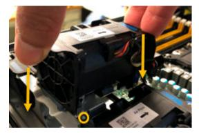
**7.** Press the fan's connector firmly into the circuit board.
