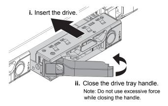
7. Insert the replacement drive in the slot, and then close the drive handle.
