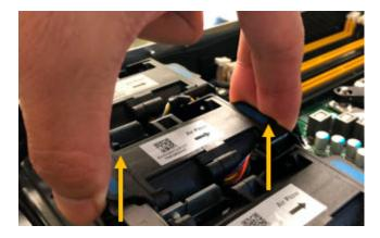
**6.** Slide the replacement fan into the open slot in the chassis. Line up the edge of the fan with the guide pin. The pin is circled in the photograph.
