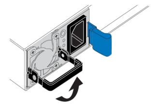
3. Press the blue latch and pull the power supply out.
