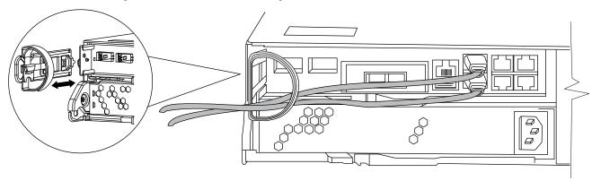
**4.** Squeeze the latch on the cam handle until it releases, open the cam handle fully to release the controller module from the midplane, and then, using two hands, pull the controller module out of the chassis.
