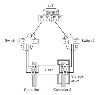
In this invalid scenario, Connection 3 from 0a through Switch 1 is incorrectly zoned to both Connection 4 and Connection 5. Likewise, Connection 3 from 0c through Switch 2 is incorrectly zoned to both Connection 4 and Connection 5. The result is that array LUN 1 is seen over more than two paths.
