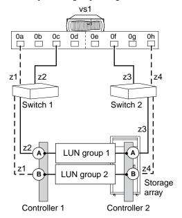
This multiple LUN group configuration enables you to spread the I/O across the RAID groups (parity groups) on the storage array. You set up your configuration so that different V-Series FC initiator
