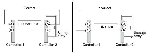
The storage errors show command shows the array LUN that is in the same fault domain. You can also see this problem in the storage disk show output if you look at the TPGN column (Target port group number). A different TPGN should be shown for each initiator in an initiator port pair. If the TPGN is the same for both initiators in the pair, both initiators are in the same fault domain.
