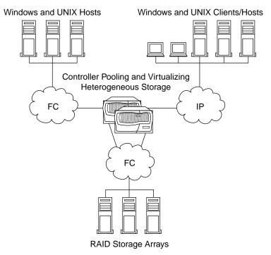
A V-Series system presents storage to clients either in the form of Data ONTAP file system volumes, which you manage on the system by using Data ONTAP management features, or as a SCSI target that creates LUNs for use by clients. In both cases (file system clients and LUN clients), on the V-Series system you combine the array LUNs into one or more Data ONTAP volumes for presentation
