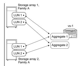
**Note:** This example is not supported if you have storage arrays of the same model and one has Fibre Channel drives and the other storage array has SATA drives. In that case, those storage arrays are not considered to be in the same family.
