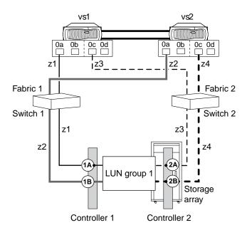
In this configuration with a single 4-port LUN group, array LUNs are mapped to four ports on the storage array. The array LUN group is presented to both nodes in the HA pair on different array target ports. However, each V-Series system can see an array LUN, end-to-end, through only two paths. Zoning is configured so that each FC initiator port on a V-Series system can access only a single target array port.
