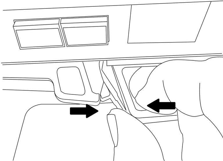
5. Turn the controller module over and open it by sliding the blue tabs to release the cover, and then swing the cover up and open.
