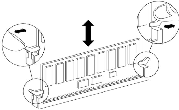
**Attention:** You must carefully hold the DIMM by the edges to avoid pressure on the components on the DIMM circuit board.
