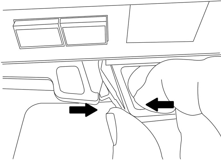
5. Turn the controller module over and open it by sliding the blue tabs to release the cover, and then swing the cover up and open.
