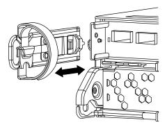
**4.** Squeeze the latch on the cam handle until it releases, as shown in the following illustration. Open the cam handle fully to release the controller module from the midplane, and then, using two hands, pull the controller module out of the chassis.
