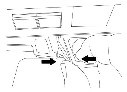
5. Turn the controller module over and open it by pressing the button to release the cover, and then slide the cover out.
