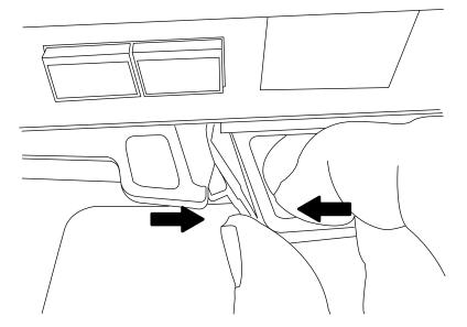
5. Turn the controller module over and open it by pressing the button to release the cover, and then slide the cover out.
