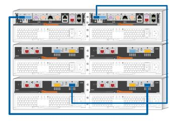
The following example displays the last set of controller-to-shelf cabling with DS4246 disk shelves:
