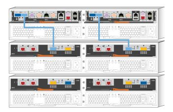
The following example displays the first set of controller-to-shelf cabling with DS4246 disk shelves:
