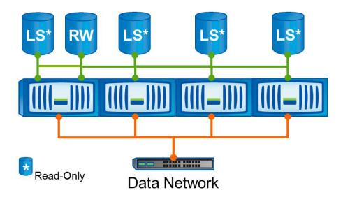
When a client requests access to a volume configured with a set of load-sharing mirrors, Data ONTAP directs all client connections only to the load-sharing mirror destination volumes. The set of load-sharing mirrors you create for the Vserver root volume should therefore include a load-sharing mirror on the same node where the source volume resides.
