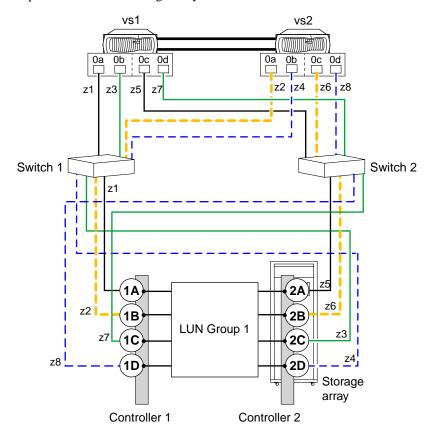
**Note:** The following problem can occur with Active-Passive storage arrays in crossed back-end connections: If one of the fabric switches is taken offline or goes down and a path failure from both Data ONTAP systems occurs, the Data ONTAP systems panic even though the alternate path from each system is still online. For example, if switch 2 is down and the "0b" paths on both vs1 and vs2 go down, vs1 and vs2 panic even though the "0a" paths are still online.
