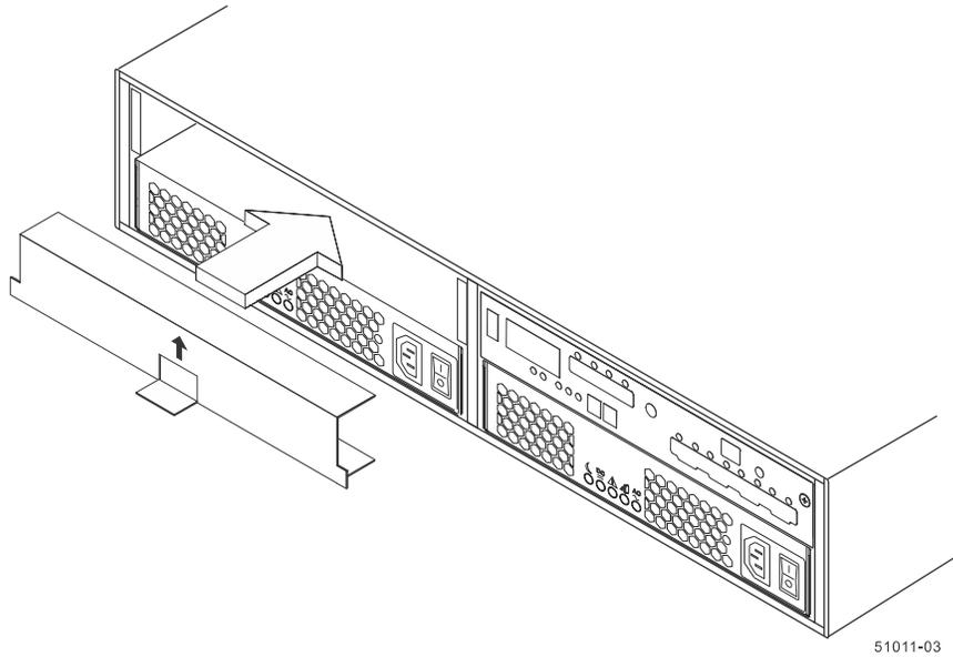
15. Remove the battery from the failed controller canister by performing these steps:
