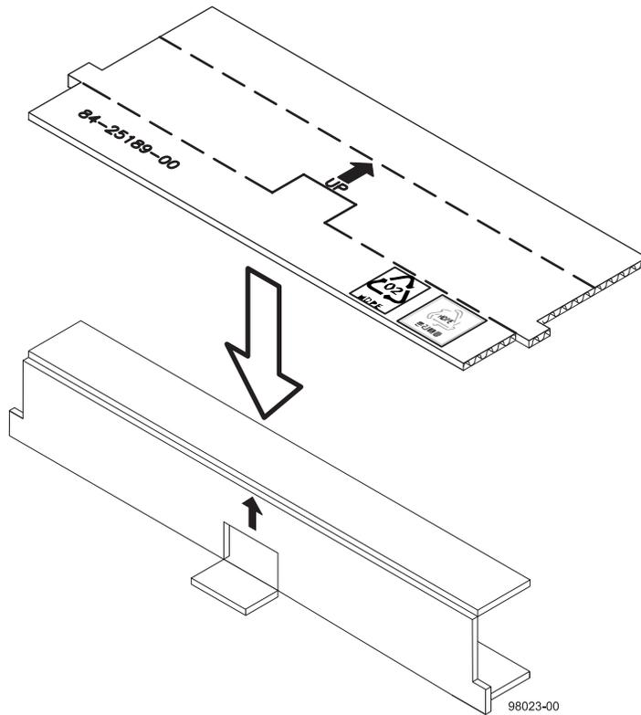
13. Remove the failed controller canister.
