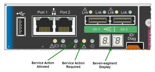
The decimal points on the seven-segment display are not used by the StorageGRID Webscale appliance:
