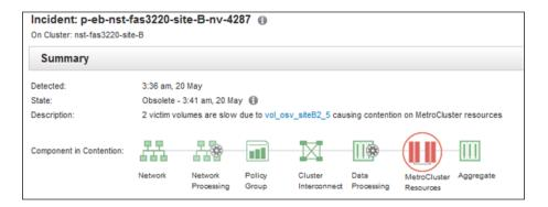
In this example, the MetroCluster Resources icon is red, indicating that the MetroCluster resources are in contention. You position your cursor over the icon to display a description of the icon. At the top of the page, **On Cluster** displays the name of the cluster on which the incident was detected.
