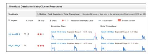
In this example, one bully workload is displayed at the top of the table. The presence of bully workloads indicates that the incident might have been caused by one or more workloads on the local cluster overutilizing the MetroCluster resources.
