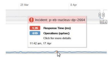
In this example, an incident is indicated by a red dot ( on the Response Time chart on the Volume Details page. Hovering your mouse cursor over the red dot displays a popup with more details about the incident and options for analyzing it.
