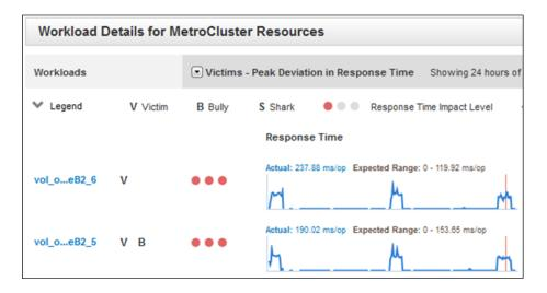
In this example, the victim workloads are displayed at the top of the table. The Response Time charts display, at a high-level, a consistent response time pattern for the victim workloads
